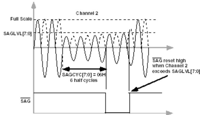
As shown in the figure above, when the instantaneous effective value of the voltage is less than the threshold set in the drop voltage threshold register (SAGLVL) and the drop time exceeds the set time in the drop line period register (SAGCYC) (the figure shows after the sixth half cycle is exceeded, SAGCYC[11:0]=06H), the line voltage drop event is recorded by setting the SAG flag bit in the interrupt status STATUS1 register
