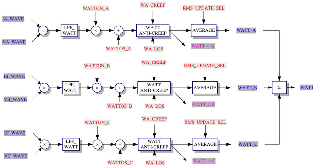
The three-phase current and voltage waveforms are respectively digitally multiplied, and then passed through the low-pass filter, gain and deviation calibration, anti-creeping judgment and averaging in order to obtain the split-phase power signal, which is added to obtain the total active power.
