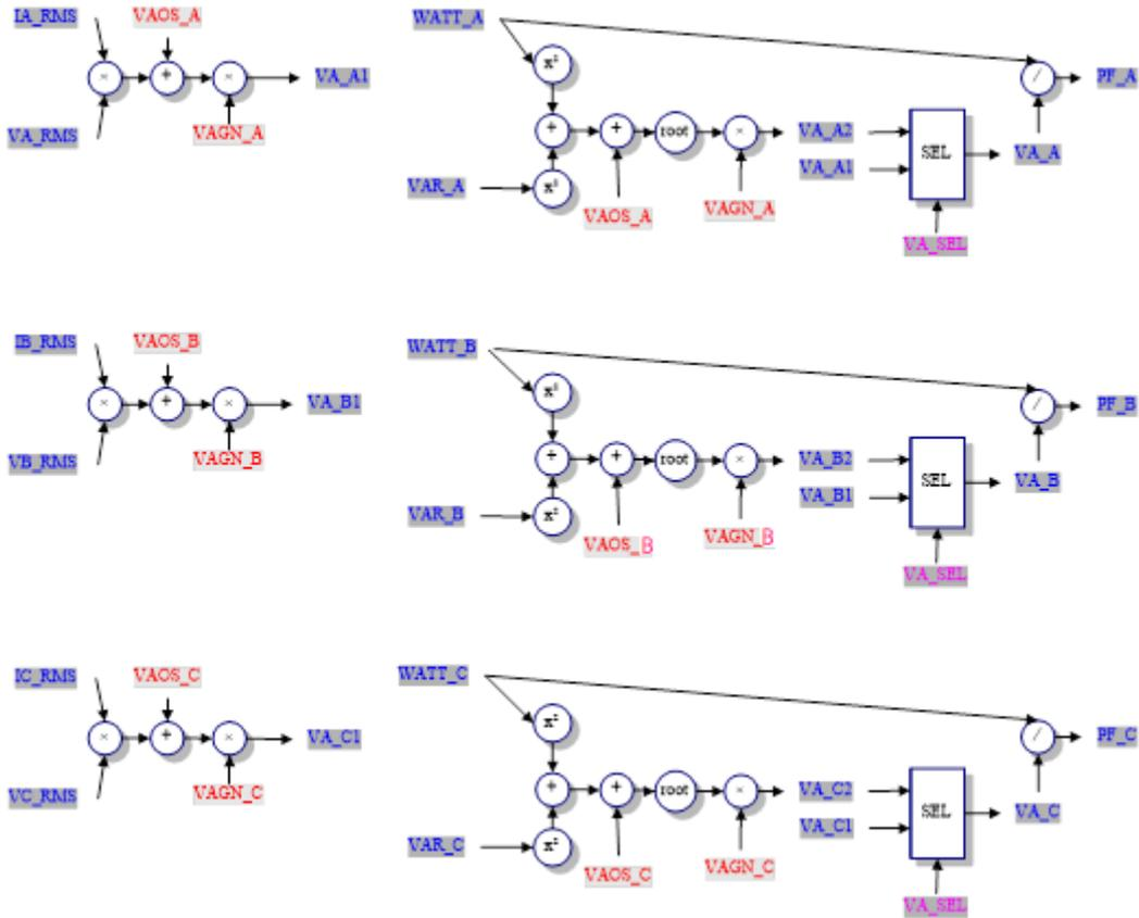
There are two ways of apparent calculation: One is the digital multiplication of the effective value of the current and voltage, and then the apparent power signal can be obtained after gain and offset calibration. The active power is divided by the apparent power to obtain the power factor.
