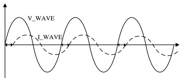
The phase difference is obtained by calculating the time difference between the positive phase zero crossing of the current and the voltage, and the corresponding time value is updated to the register CORNER[N]. Each register is a 16-bit unsigned number.
