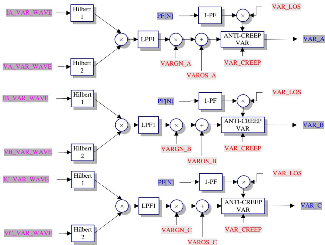
After the current and voltage waveforms of each phase pass through the Hilbert filter, digital multiplication is performed, and then the reactive power signal can be obtained after the low-pass filter, gain and deviation calibration, anti-creeping judgment and averaging processing in order. After integration, the reactive energy pulse accumulation is obtained.
