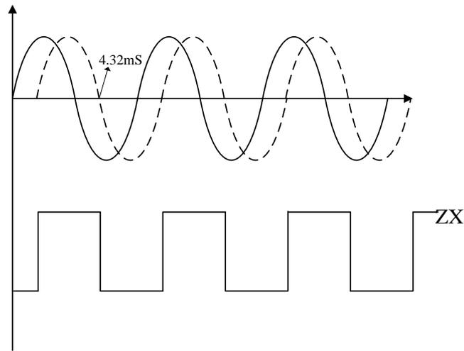
Note: In order to prevent the uncertainty caused by the presence of noise signals or spurious signals in the presence of small signals, the current zero-crossing threshold is 70,000, and the voltage zero-crossing threshold is 200,000. If the instantaneous effective value is smaller than the threshold, there is no ZX signal.
