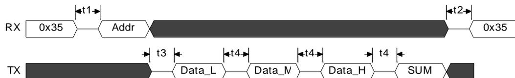
The host UART read data sequence is shown in the figure below. The host first sends the command byte (0x35), then the address byte (ADDR) that needs to be read, then BL6552 sends the data byte in turn, and finally the checksum byte.
