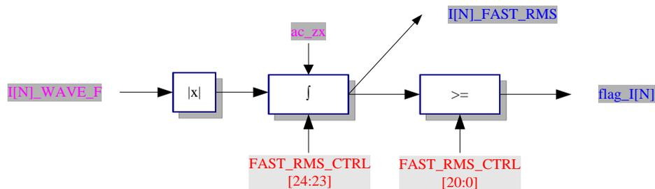
7 channels have fast effective value registers, which can detect half cycle or cycle effective value. This function can be used for overcurrent detection.
