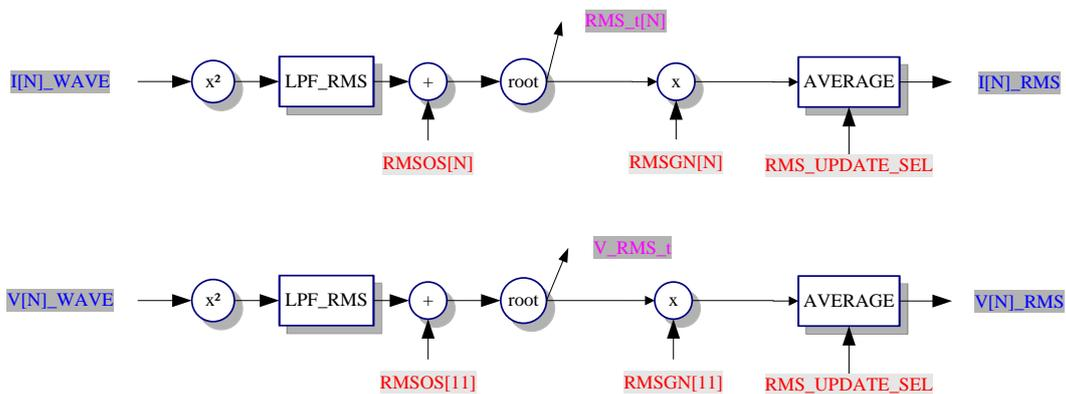
The original waveform of each channel passes through the square circuit ( $X^2$ ), the effective value low-pass filter (LPF\_RMS), and the root circuit (ROOT) to obtain the instantaneous value RMS\_t of the effective value, and then average the average value of each channel The values I[N]\_RMS and V[N]\_RMS.
