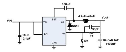
*Notice:* BL9362 minimum duty cycle = 20%, and the relationship between duty cycle to output voltage and input voltage is duty cycle = output voltage / input voltage, so the maximum input voltage = output voltage / 0.2 to ensure that SW does not cause frequency hopping due to too small duty cycle.
